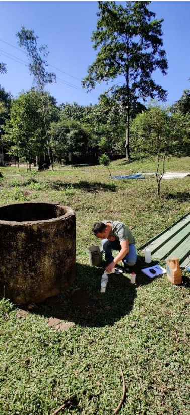
Water level measurement from dug well and water sample collection in South Garo Hills district
